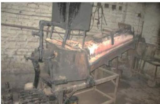
Conventional furnace in a hand tool unit
